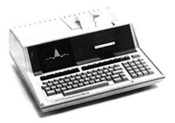
A powerful BASIC language computer complete with built-in keyboard, CRT display, printer, tape unit, and graphics system.
